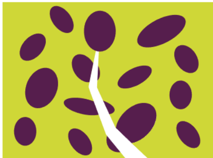
Microcapsules ruptured by fracture
