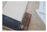
To make measuring my pieces of wood accurate as possible I used gauge and a tri square the gauge was used to make parallel lines to an edge and the tri square was used to make 90degrees angle accurately.
