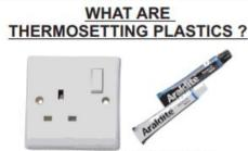
www.technologystudent.com Once heated and moulded, these plastics cannot be reheated and remoulded. The molecules of these plastics are cross linked in three dimensions and this is why they cannot be reshaped or recycled. The bond between the molecules is very strong.
