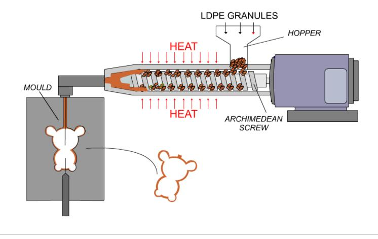
The extrusion blow moulding process (EBM), is very similar to <u>blow moulding</u>. The only difference is at the mould.
