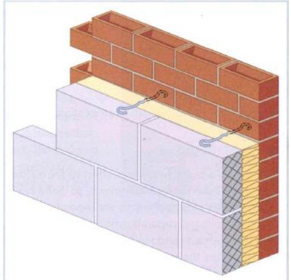
Find out exactly where a bricklayer should place their walls ties when constructing a cavity wall
