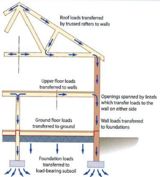
Figure 1.1 A dynamic load is transferred from the roof to the foundations through the walls and floors
